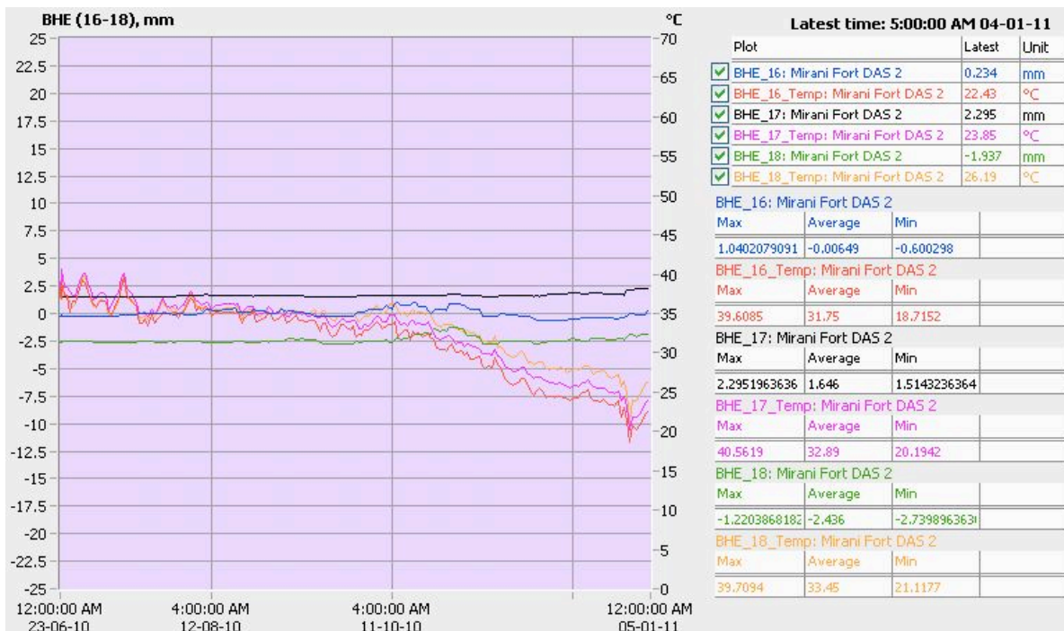
Figure 11 – screen shot of data from a borehole extensometer
