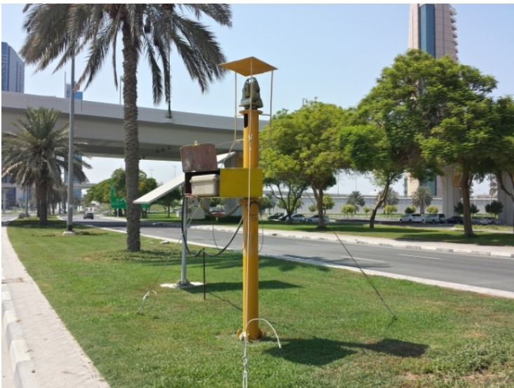
Figure 2: Installed ATS on site with control box and solar panel power supply
