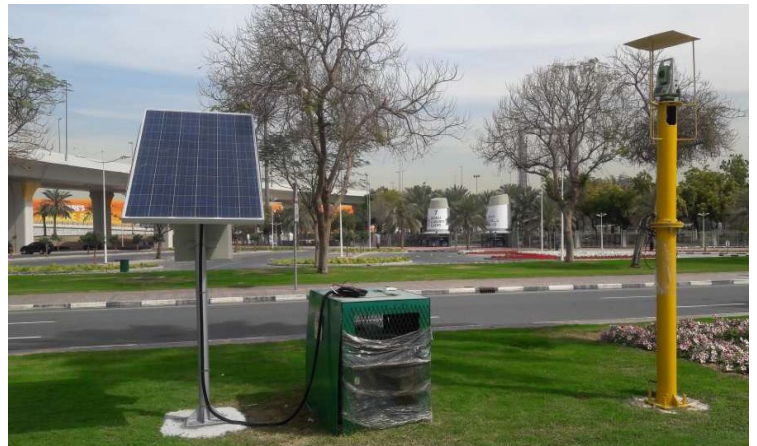
Figure 9 Prism target locations on the bridge pier (left). Automatic total station to collect and transmit data from prism targets installed on bridge (right)
