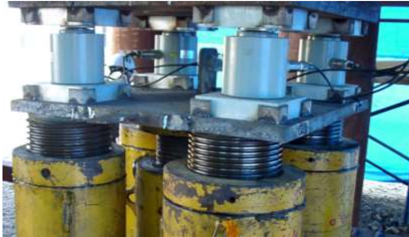
Figure 4.3 Pile load testing
