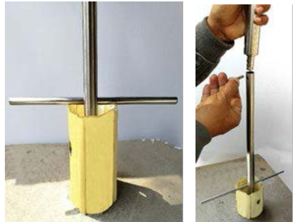
Figure 7: Inserting retaining rod in the spacer tubing
