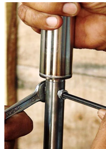
Figure 8: Fixing sensor to spacer tubing
